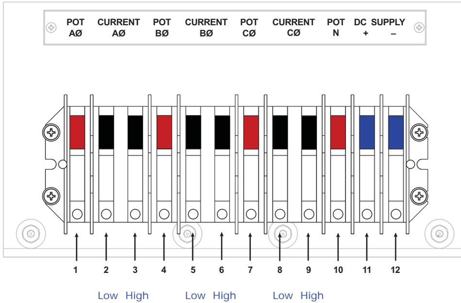
Figure 13.4: Detail of Test Switches
