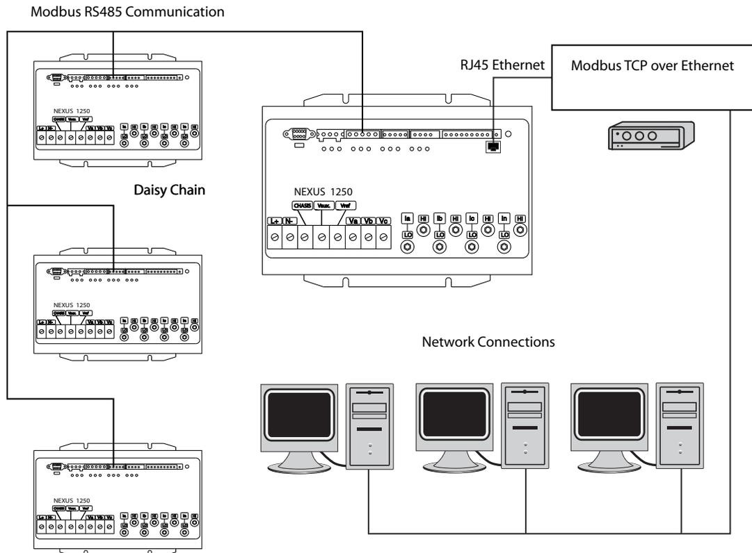
Figure 11.1: Meter Communication with Network Option/Daisy Chained Meters
