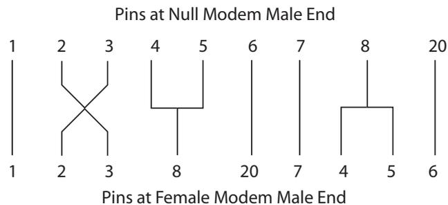
Figure 5.10: Standard Null Modem Configuration
