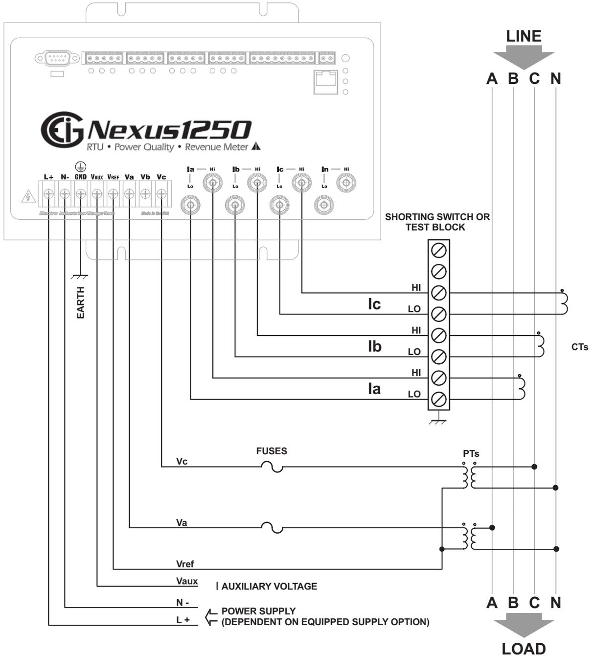
Figure 4.8: 3-Phase, 4-Wire, 2.5 Element with 2 PTs and 3 CTs
