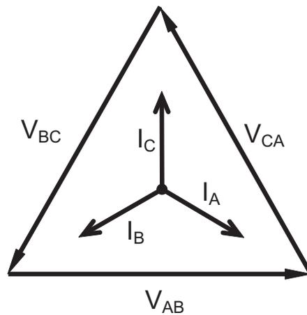
Figure 1.4: Phasor Diagram, Three-Phase Voltages and Currents, Delta-Connected
