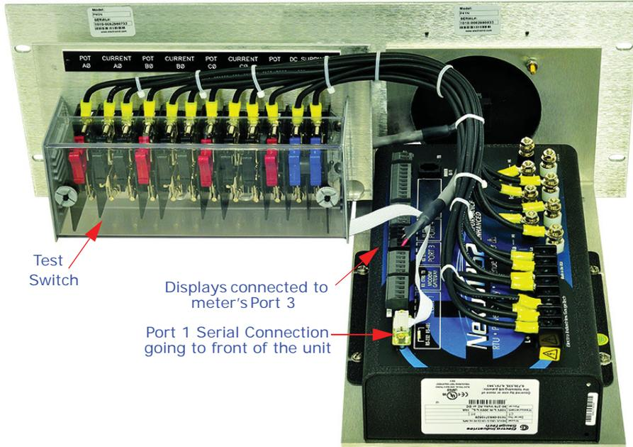
Figure 13.3: Back of Rack Assembly
