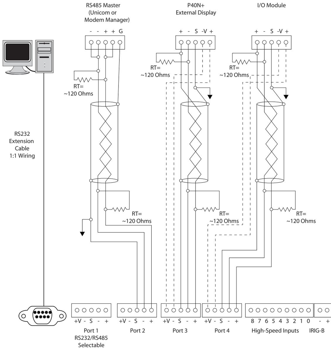
Figure 5.3: Communication Wiring
