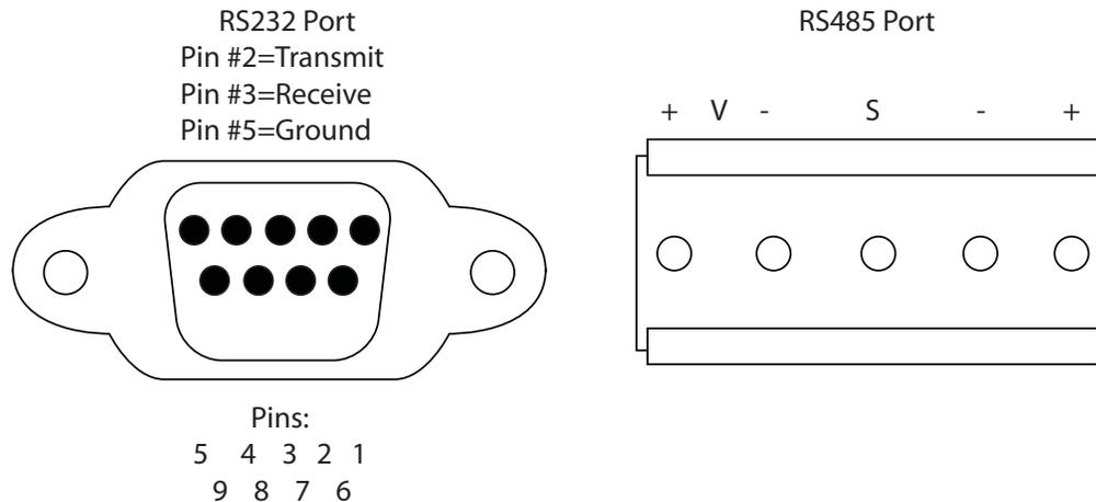
Figure 5.4: RS232/RS485 Port Detail
