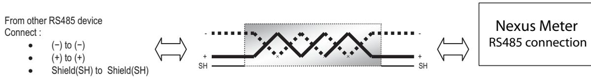
Figure 5.5: 2-Wire RS485 Port Detail
