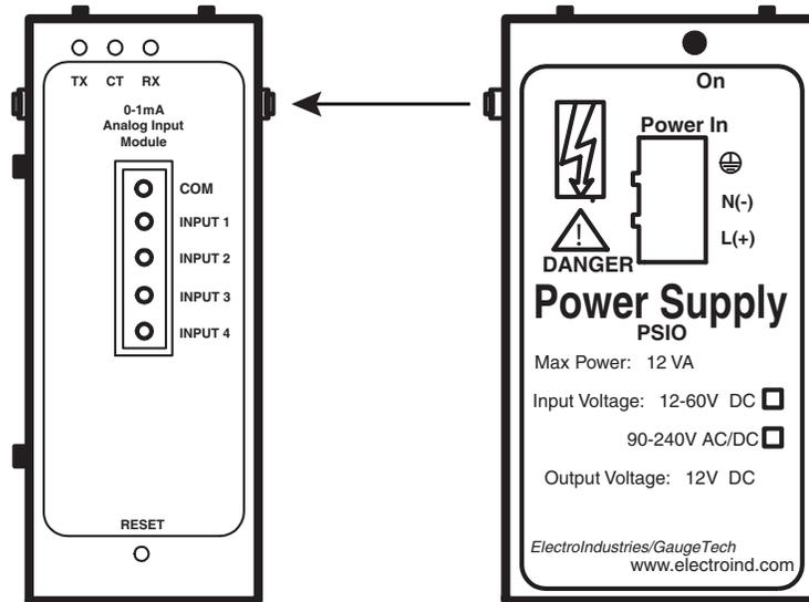
Figure 9.3: Power Flow from PSIO to I/O Module
