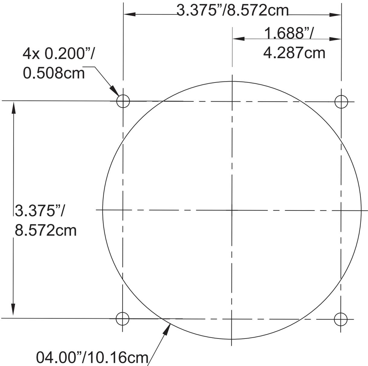
Figure 3.4: ANSI C39.1 Drill Plan for P40N/P40N+ Display
