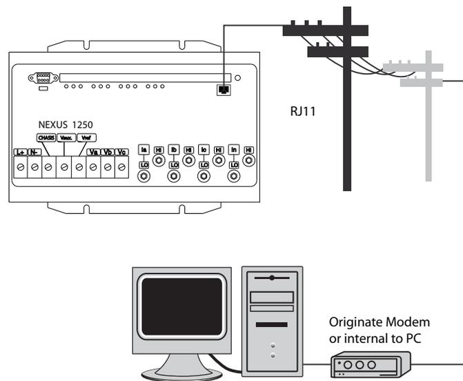
Figure 10.1: Meter Communication with Internal Modem Option
