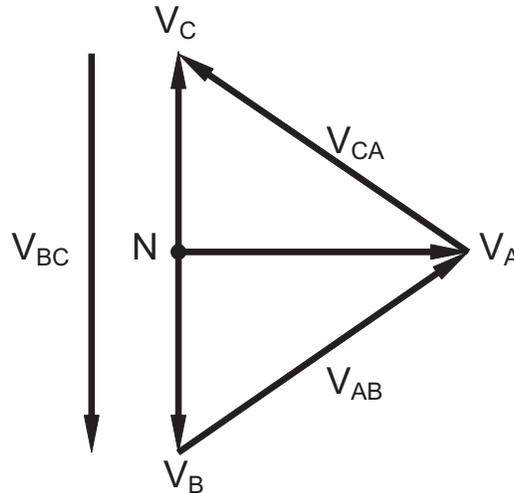
Figure 1.5: Phasor Diagram Showing Three-phase Four-Wire Delta-Connected System
