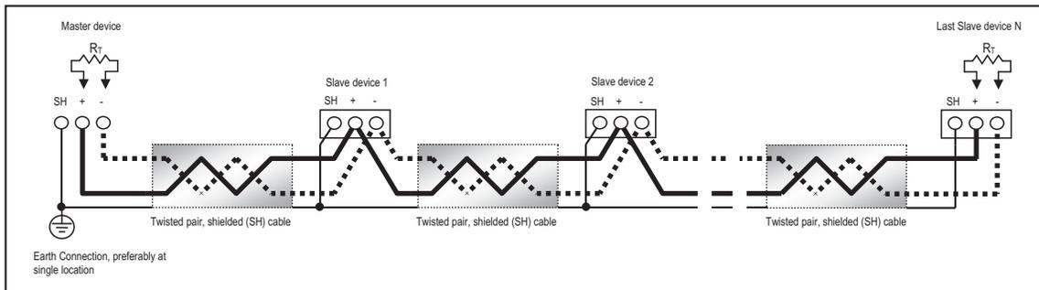
Figure 5.9: Linking Multiple Nexus® Meters in Series
