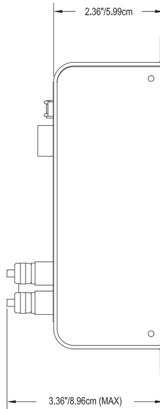
Figure 3.2: Nexus® 1250/1252 Mounting Diagram Side View
