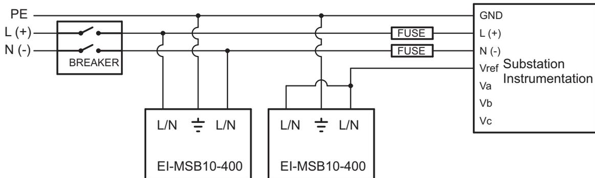
Figure 4.10: Wiring Schematic for Extended Surge Suppression
