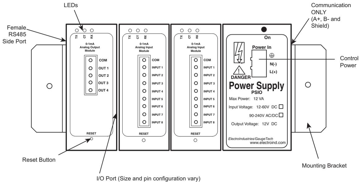
Figure 9.5: PSIO Used with Multiple I/O Modules
