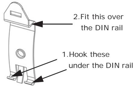
Figure 9.7: Detail of DIN Rail Mounting Clip
