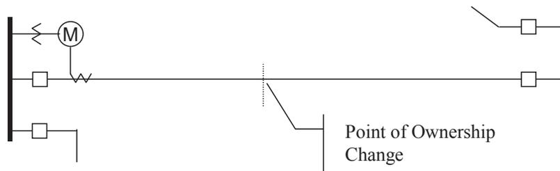
Figure 7.2: Joint Ownership Line Meeting Requiring Loss Compensation
