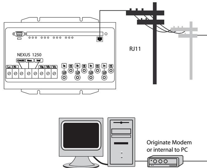
Figure 5.1: RJ11 Communication with Internal Modem Option
