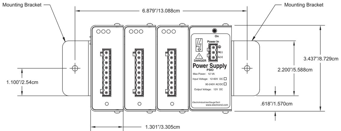
Figure 3.7: I/O Modules Mounting Diagram Front View
