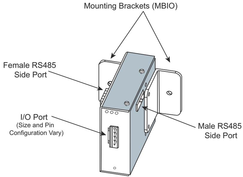
Figure 3.6: I/O Module Communication Ports and Mounting Brackets
