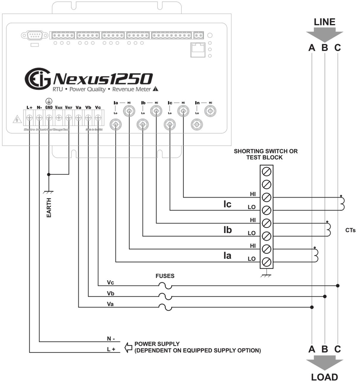
Figure 4.7: 3-Wire, 2-Element Delta Direct Voltage with 3 CTs
