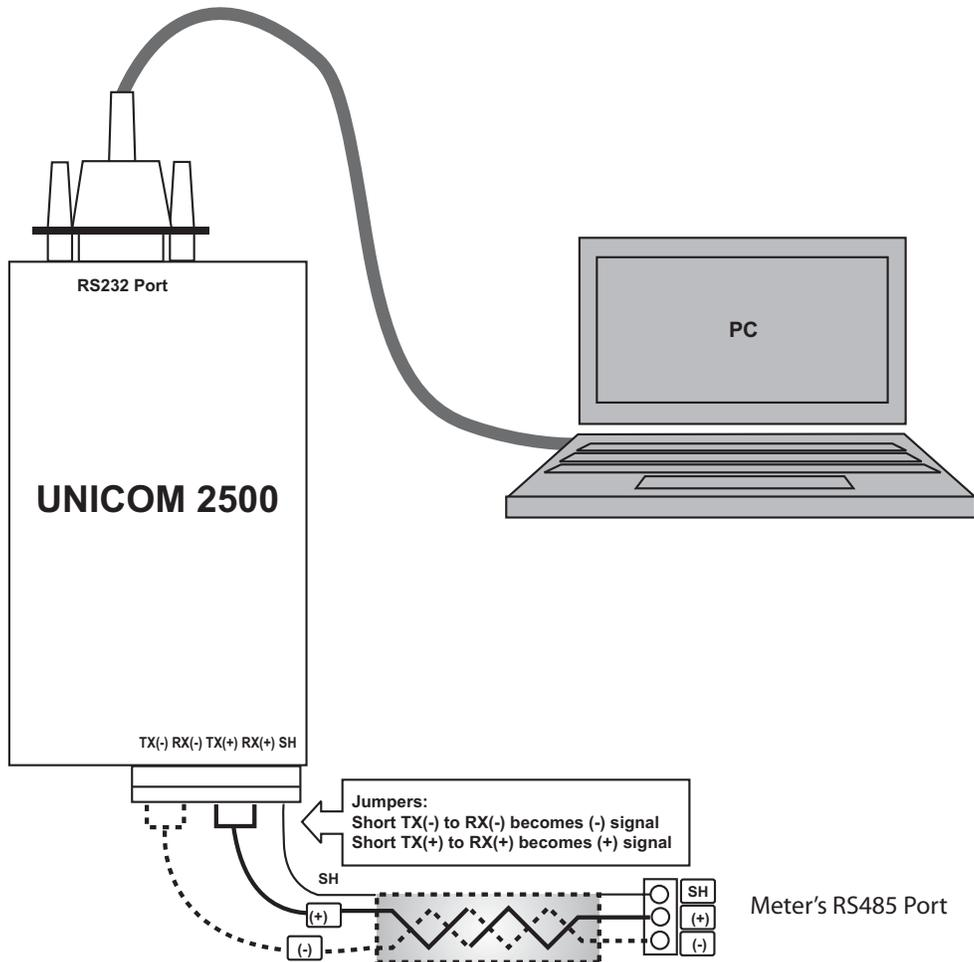
Figure 5.7: Meter Connected to PC using Unicom 2500
