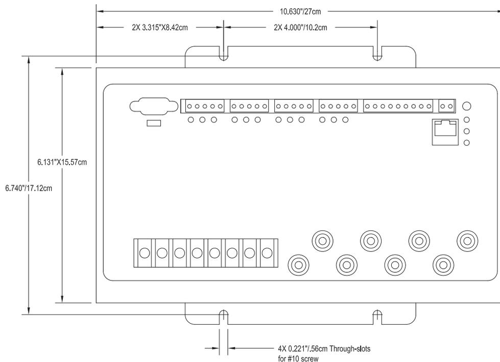
Figure 3.1: Nexus® 1250/1252 Mounting Diagram Top View
