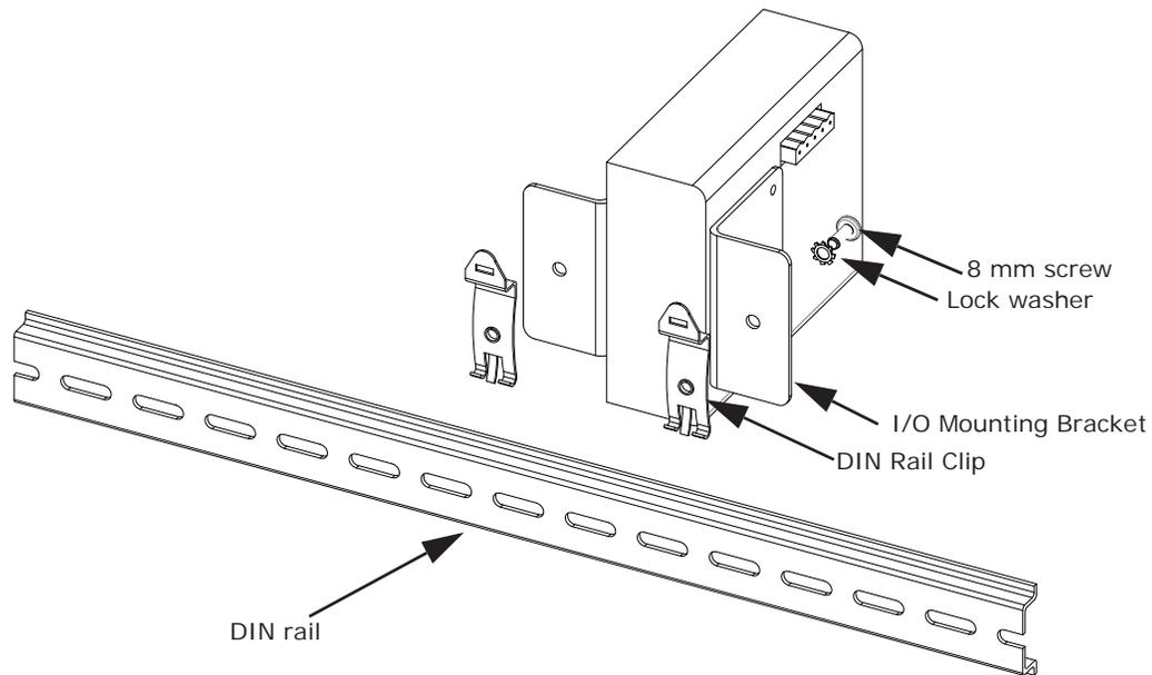
Figure 9.6: Mounting the Brackets on a DIN Rail
