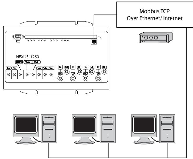
Figure 5.2: RJ45 Communication with Internal Network Option
