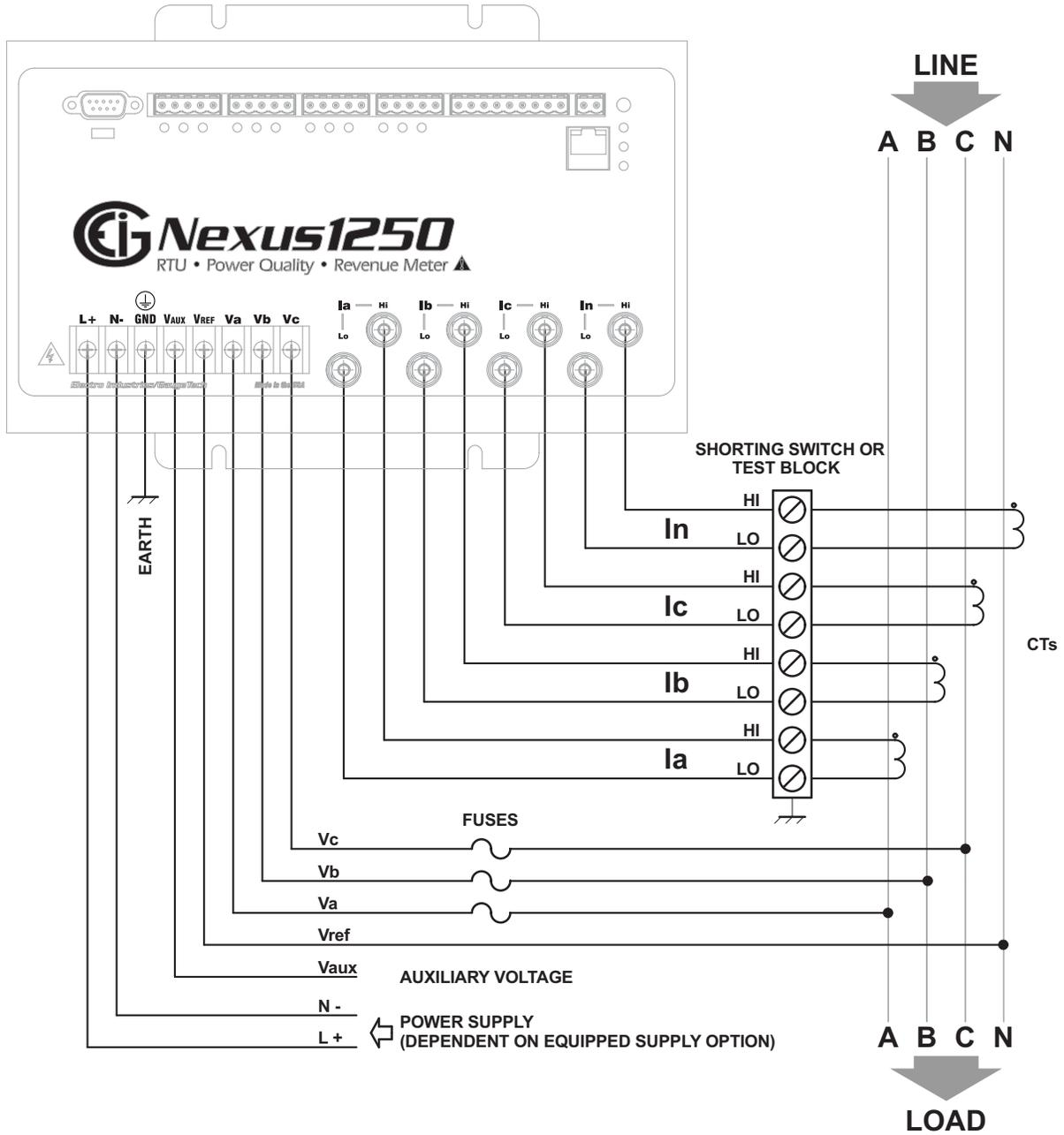
Figure 4.2: 4-Wire Wye, 3-Element Direct Voltage with 4 CTs
