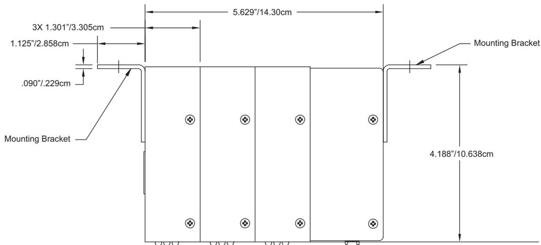
Figure 3.5: I/O Modules Mounting Diagram Overhead View
