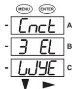
9. Press the **ENTER** button to go to the Scroll setting screen (SCrL). The current setting is shown in the second line. Press the **DOWN ARROW** to choose another setting. You can choose YES (the meter readings will scroll on the display) or no (the meter readings will not scroll on the display).
