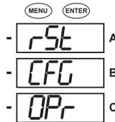
2. Press the **DOWN ARROW** once. CFG (Configuration) moves to the top of the display.
