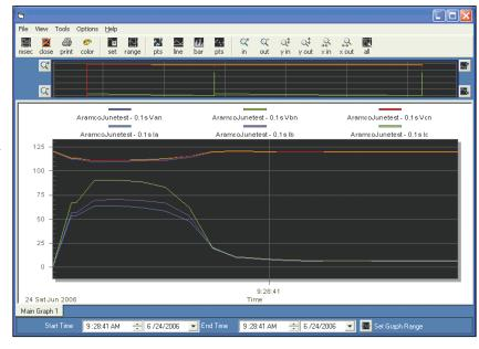
The screen shows the TRMS value recording chart for voltage and current.
