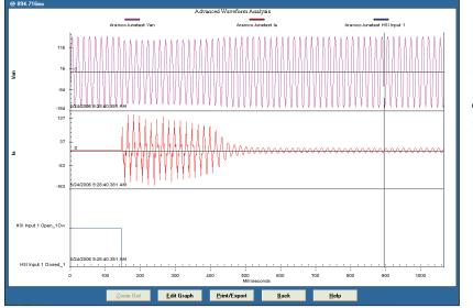
The screen shows a typical motor startup waveform reading.
