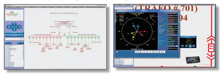
EIG SCADA HMI EXT sample screens: Single line Master systems diagram screen
